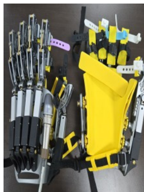
(b) Exoskeleton hand brace
