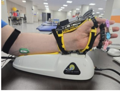
(a) EMG sensor on the finger flexor muscle
